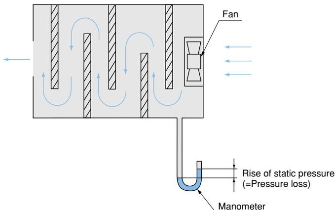
Fig. 2 Flow path with high air flow resistance
