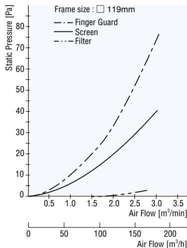
Fig.8 Pressure loss due to optional parts
