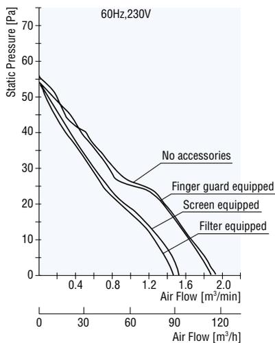
Fig.9 Changes in characteristics with optional parts attached to the **MU1225S-51**
