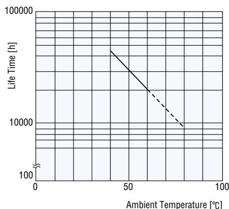
Fig. 13 Characteristic curve for estimating life
