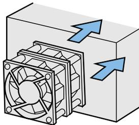
Fig.5 Installing two fans in series
