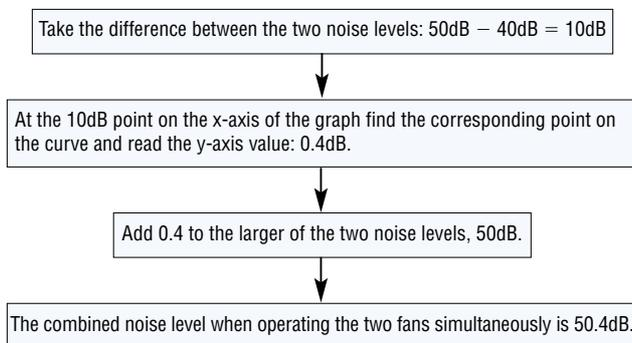
If 40dB of noise is combined with 50dB, the resulting increase in noise is only 0.4dB. Thus, when fans of different noise levels are operated simultaneously, it is more important to reduce noise from the fan with the higher noise level.
