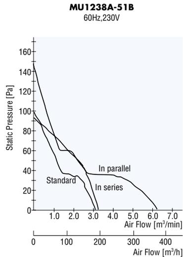
Fig.7 Characteristics for different installation methods
