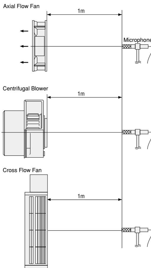
Fig.10 Measurement of fan noise.
