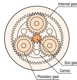
Cross section of a **PL** gear
