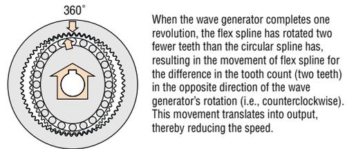
When the wave generator completes one revolution, the flex spline has rotated two fewer teeth than the circular spline has, resulting in the movement of flex spline for the difference in the tooth count (two teeth) in the opposite direction of the wave generator's rotation (i.e., counterclockwise). This movement translates into output, thereby reducing the speed.
