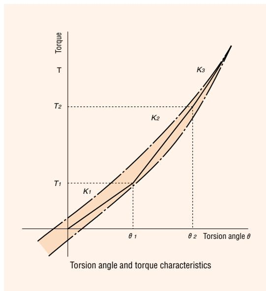
Torsion angles obtained by these equations are for individual harmonic gears.
