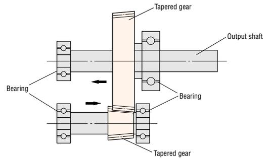
Structure of **TH** gear's final stage
