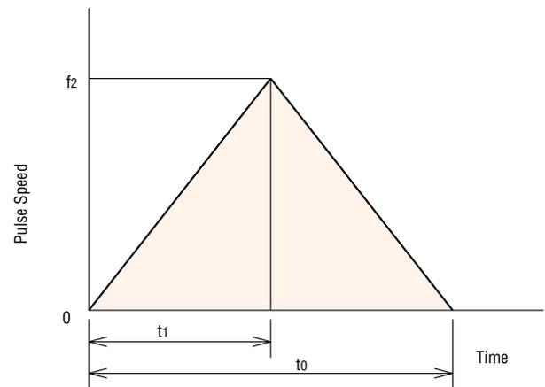
If the pulse velocity is  $f_2$ , the positioning time  $t_1$ , the operation pulse count A, and the acceleration rate  $T_r$ , then the following equation holds.
