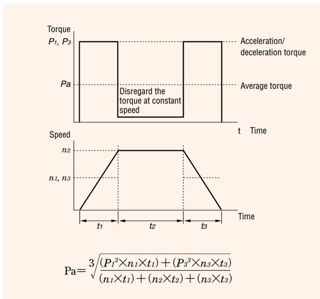
◇ **Driving an Inertial Body Only ② : Driving an Arm or Similar Object**
