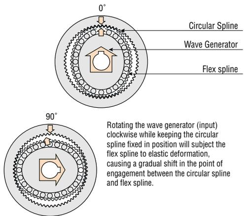
Combines three basic parts. The flex spline is bent into an oval shape by the wave generator. The teeth at the long axis of the oval mesh with the circular spline, while the teeth at the short axis of the oval are completely separate from it.
